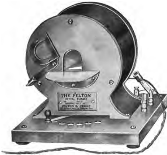
Pelton electrical furnace.
